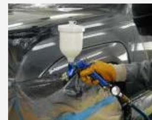
Note, **Toyota HS Multi Surfacer** can be used as a wet-on-wet primer or as Sanding Surfacer.
