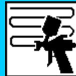
Apply 1 light coat on fade-out-zone @ 0.8 - 1.5 bar
